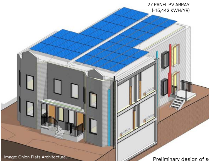
Preliminary design of solar PV array.
