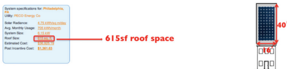
figure 14.3. Required roof area for 4.5 kWh/sf/year consumption
